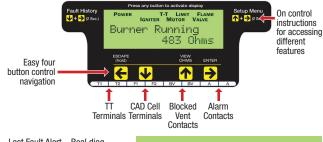
Last Fault Alert – Real diagnostics that spell out what the problem is when your technician arrives on the job even if control has been reset. At the right is a snapshot of what you could see on a no heat call.
