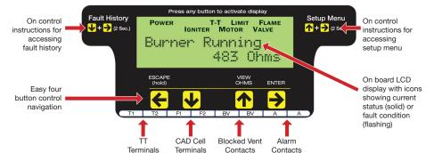
Last Fault Alert – Real diagnostics that spell out what the problem is when your technician arrives on the job even if control has been reset. Below is a snapshot of what you could see on a no heat call.
