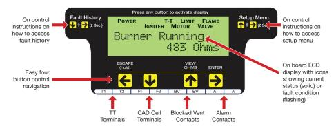
Last Fault Alert – Real diagnostics that spell out what the problem is when your technician arrives on the job even if control has been reset. Below is a snapshot of what you could see on a no heat call.
