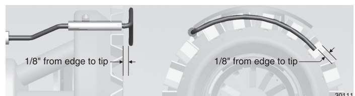
Figure 7 Flame rod location
