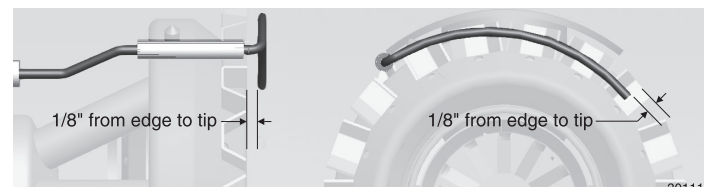
Figure 7 Flame rod location
