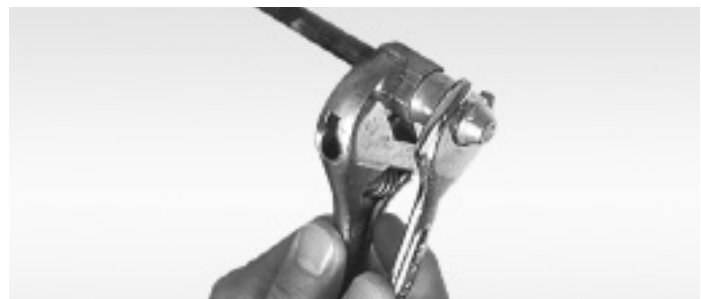
Figure 3 Carefully support the nozzle adapter when removing or installing nozzle
