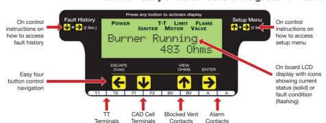
Last Fault Alert – Real diagnostics that spell out what the problem is when your technician arrives on the job even if control has been reset. Below is a snapshot of what you could see on a no heat call.
